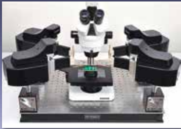
Installation example for 4-terminal measurements
