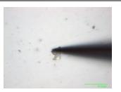
Picking up and transferring 5µm toner (using 5 micron glass probe)
