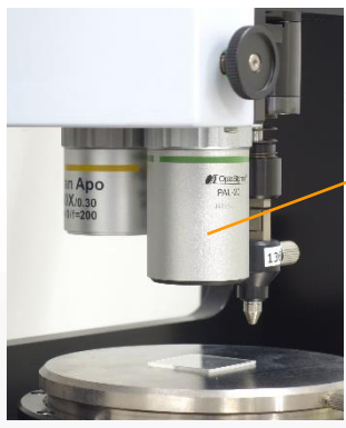
【Objective lens】 Up to two objective lenses can be mounted and used interchangeably
