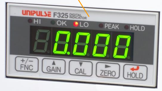
【Load Measurement Capability】 Comes standard with a sensor adjustable from as low as 0.0005N.
