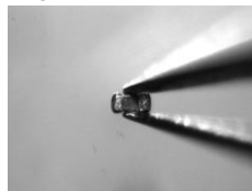
Gripping a 100μm electrical chip
