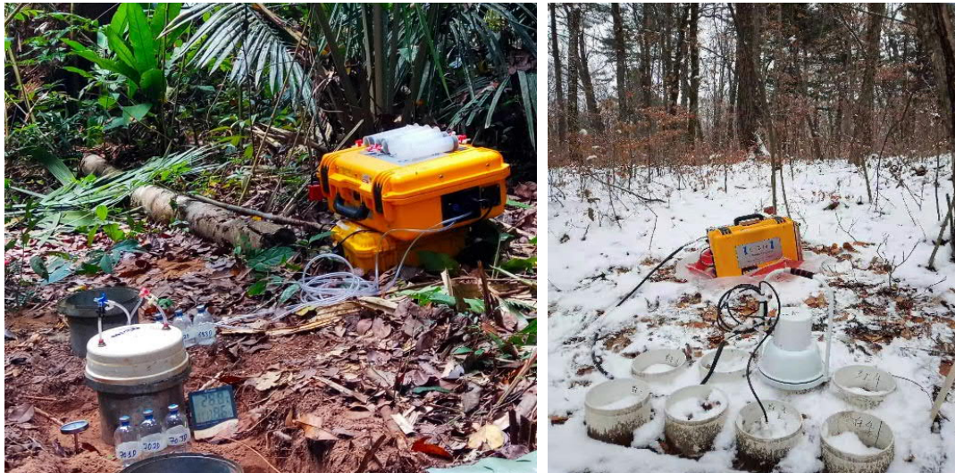
Application examples of LGR-ICOS instruments for soil flux applications. Left: in Amazonia (Courtesy Wanderlei Bieluczyk, USP-CENA), right: in Chinese forest (Courtesy Lica United)
